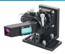
This motorized variable attenuator/beamsplitter consists of special design opto-mechanical Adapter and precision opto-mechanical holder 840-0193. Two Thin Film Brewster type polarizers, which reflect s-polarized light while transmitting p-polarized light, are housed into Adapter. Quartz Half Waveplates are housed in motorized rotation stage 960-0161.
